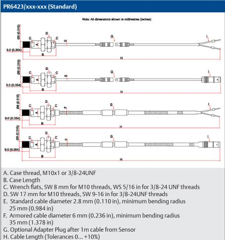
I. Lemo connector (male), 11.0 mm (0.433 in) diameter or open cable end
